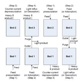
Figure 1: A two-bed four-step PSA cycle
