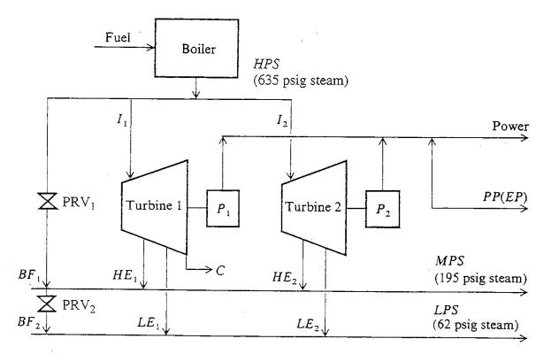
Figure 3. Steam-power system with power generation and/or purchase (Edgar et al., 2001).
