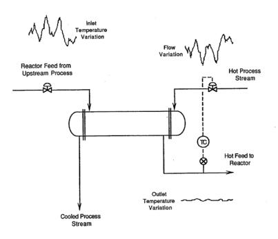
Figure 5. Transformation of variation from the temperature to flow for a reactor feed preheater (Downs et al., 1991)
