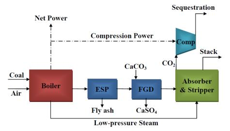
Figure 1. Absorption/Stripping as a post-combustion process for CO<sub>2</sub> capture from coal-fired power plants
