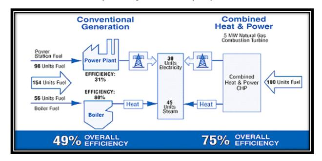
*Figure 2 Comparison of energy flows for conventional generation vs. combined heat and power (cogeneration), Source: EPA.*
