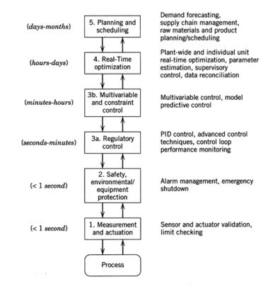
Figure 4. The five levels of process control and optimization in manufacturing. Time scales are shown for each level (Seborg et al., 2010)
