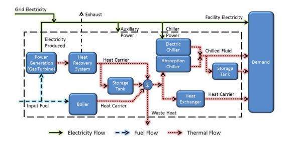
Figure 6. Schematic of CHP-TES system. The demand can be a heating and cooling network (Wang, et al., 2010)
