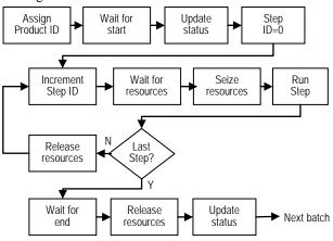
Figure 5. Generic simulation logic
