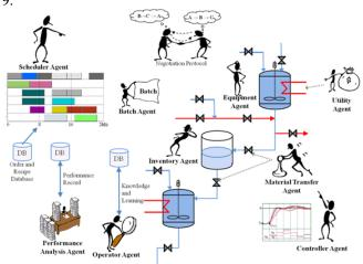
Figure 9. Agent-based real-time batch management system
