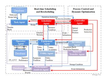
Figure 10. Expected architecture of the MAS
